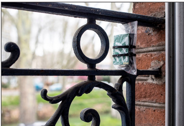
Fig. 5 — Example of installation of an AudioMoth recorder on a balcony near an urban roadway in Toulouse, France (Photograph: S. Challéat, UMR CNRS 5602 GÉODE).
