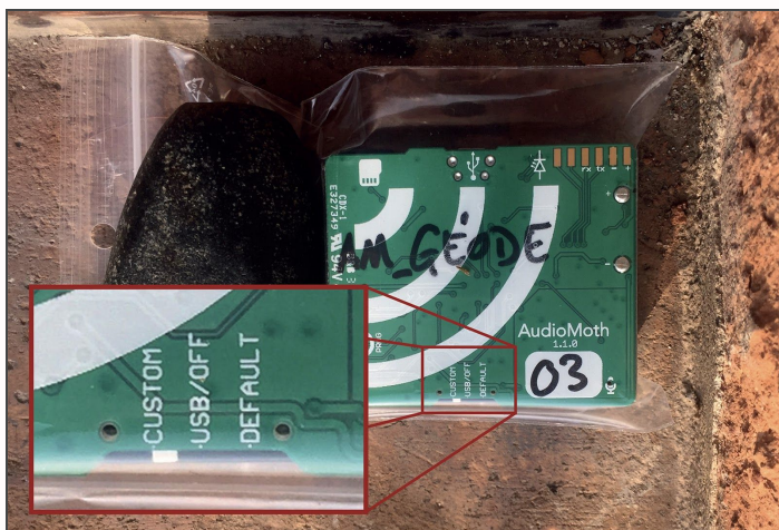
Fig. 6 — An AudioMoth recorder in a small protection plastic bag (Photograph: A. Burens, UMR CNRS 5602 GÉODE).
